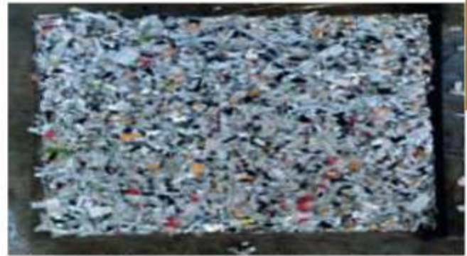
Figure 2. Pre pressed mat of tetra pack material
