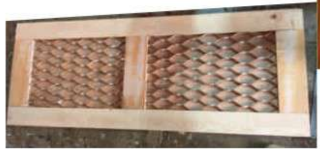
Fig. bamboo honeycomb structure placed in door framework.
